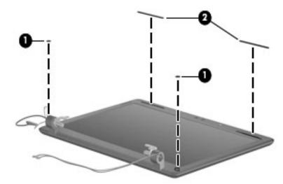
b. Remove the two PM2.0×5.0 screws **1** and two PM3.0×6.0 **2** screws that secure the display bezel to the display enclosure.
